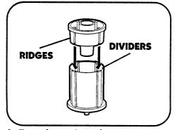
4. To re-insert base into carousel, align ridges on base with dividers on carousel, and slide base in. Tighten screw with a screwdriver.
